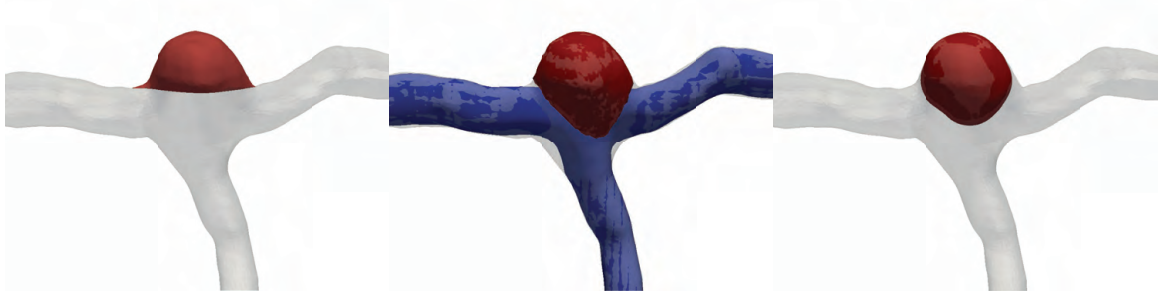
Figure 9. Planar isolation volume (red) overlaid on aneurysm geometry (gray) on left, non-planar isolation (red) overlaid with parent vessel reconstruction (blue) on parent vasculature (gray) in middle, and Voronoi diagram core volume (red) overlaid on parent vasculature (gray) on right.
